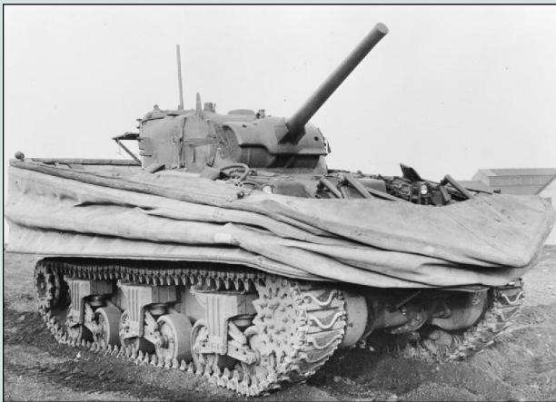
Sherman "DD" duplex drive swimming tank
